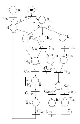
Figure 6: Mapping of Task Structure of Figure 3 to WF-net
