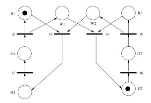
Figure 4: A Petri-net modeling two traffic lights.
