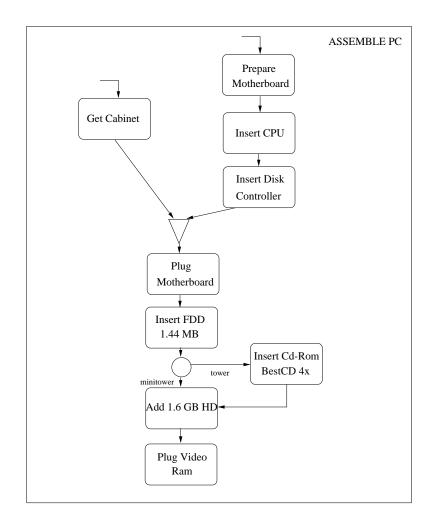
Figure 2: Main task for desktop assembly line
