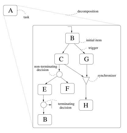
Figure 1: Graphical representation of Task Structure concepts
