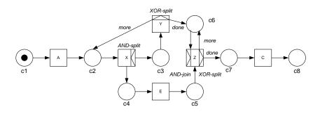
Figure 10: Multiple activation of activity B using the milestone pattern
