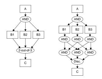
Figure 4: Implementation of 2-out-of-3-join using simple discriminator
