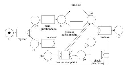
Figure 9: The state in-between the processing/time-out of the questionnaire and archiving the complaint (i.e. place  $c_4$ ) is an example of a milestone.
