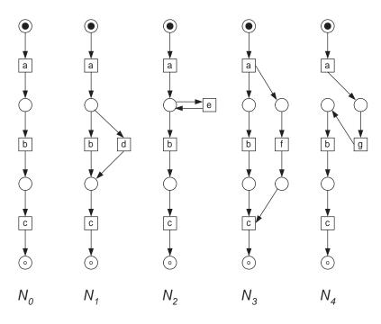
Fig. 6.  $N_2$ ,  $N_3$ , and  $N_4$  are subclasses of  $N_0$  under projection inheritance.
