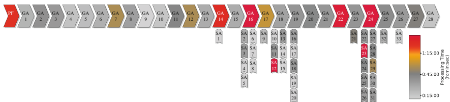
Fig. 5.8 Visualization of service time (red color scale) on the general assembly line and subassembly stations. The major bottleneck in the process is formed by the general assembly station GA16
