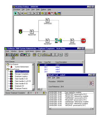
Fig. 10. The Graphical Workflow Definer, Work Queue, and Audit Trail of Staffware.
