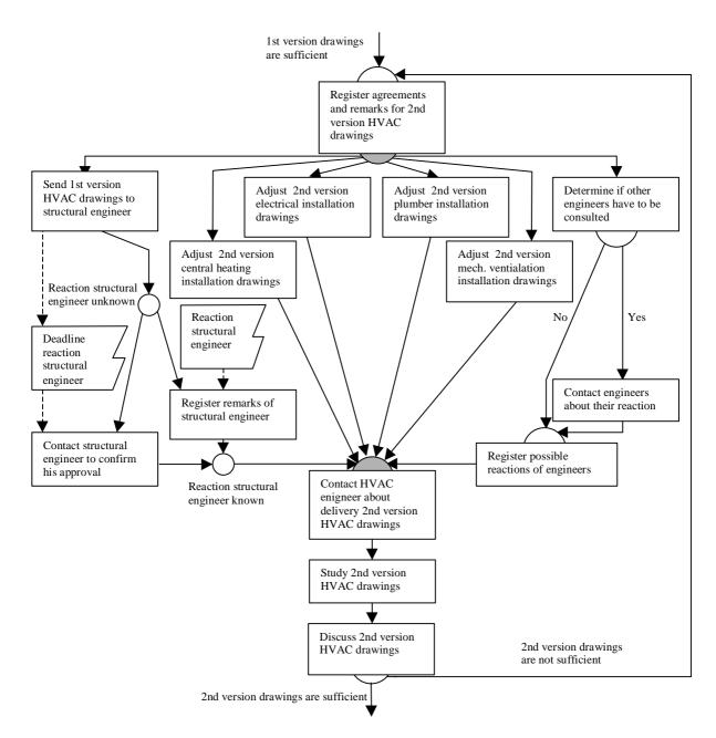
Figure 6: making of the second version HVAC drawings
