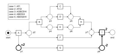
Fig. 10. Some diagnostics showing the mismatch between Figure 9(a) and event log L3.
