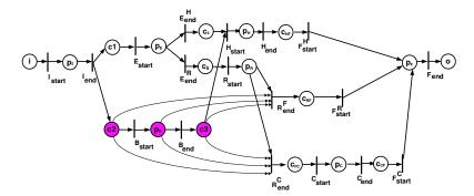
**Fig. 2.** Holiday scenario - RWF-net (Double-headed reset arcs from c2, c3 and  $p_B$  to  $R_{end}^F$  and  $R_{end}^C$ )
