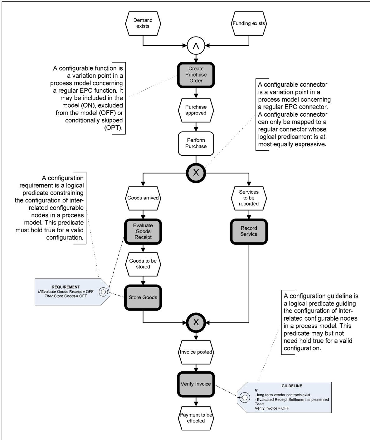
Adhering to design principle (i) C-EPCs extend regular EPCs with the specification of variation points (configurable functions and connectors), configuration requirements and configuration guidelines.
