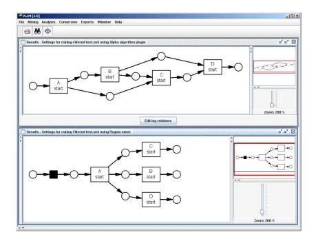
Fig. 8. A screenshot of ProM, showing the result of the  $\alpha$ -algorithm and the region approach.
