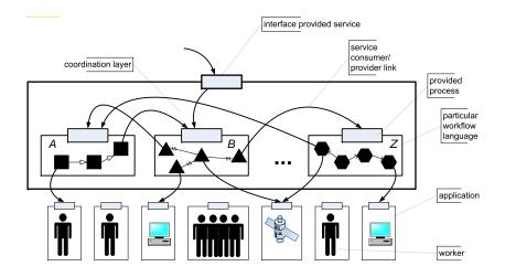
**Fig. 1.** Overview of FAAS approach:  $A, B, \ldots, Z$  may use different languages. The solid arcs are used to connect a service consumer (arc source) to a service provider (arc target).
