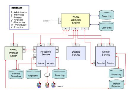
Fig. 5. High-level architecture of the YAWL environment.
