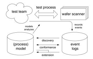
Fig. 1. Based on the event logs of the wafer scanners, three classes of process mining techniques are possible: (1) "discovery", (2) "conformance", and (3) "extension"
