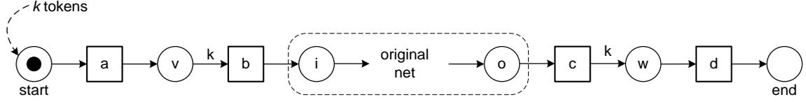
**Fig. 10.** The original WF-net is weak sound if and only if the constructed WF-net is  $k$ -sound. Because  $k$  tokens are put in place *start*, transition  $b$  fires once to initialize the original net. If the original net puts one token in  $o$ , then  $c$  can fire once followed by  $k$  executions of  $b$ , thus producing  $k$  tokens for place *end*.
