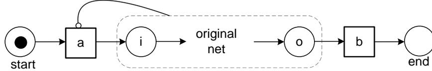
Fig. 12. The original WF-net is weak sound if and only if the constructed WF-net is generalized sound. Note that a short-hand notation is used; transition  $a$  has an inhibitor arc for each place in the original net.
