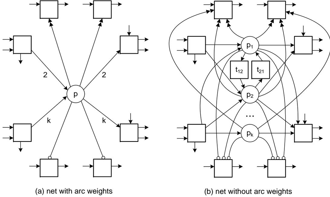
**Fig. 8.** Removing arc weights: place  $p$  is split up into  $k$  places and transitions are added such that tokens can freely move among these places. The arc weights 2 and  $k$  can be replaced by any weight  $1 \leq l \leq k$  and the construction also works for more/less input/output transitions.
