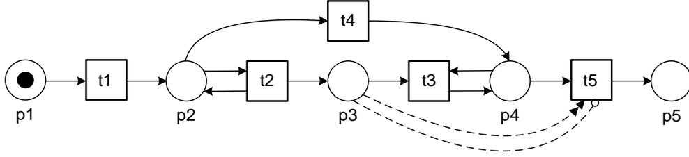
**Fig. 17.**  $N$  is the WF-net without the reset/inhibitor arc,  $N_R$  is the net with the reset arc,  $N_I$  is the net with the inhibitor arc, and  $N_{RI}$  is the net with both the reset arc and inhibitor arc.
