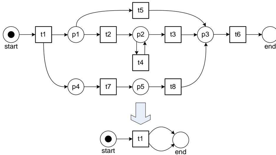
Fig. 20. A WF-net that is not sound and that cannot be reduced completely.
