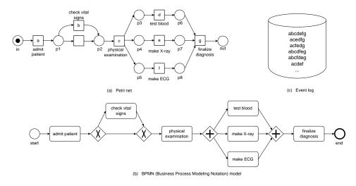
**Fig. 1.** A Petri net (a) and BPMN model (b) describing a simple medical diagnosis process. Example traces are shown in the event log (c), a = admit patient, etc.
