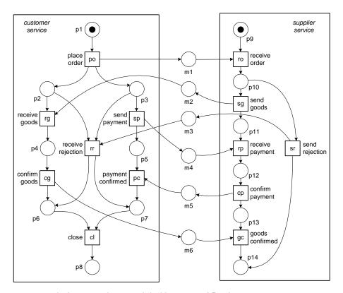
Fig. 1. A process composed of two services modeled in terms of Petri nets.
